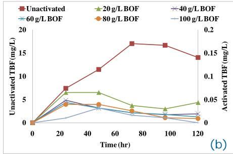
Fig. 8. Degradation of MTBE (a) and production of TBF(b) and TBA (c) during PS oxidation with the addition of different dosages of BOF slag.
