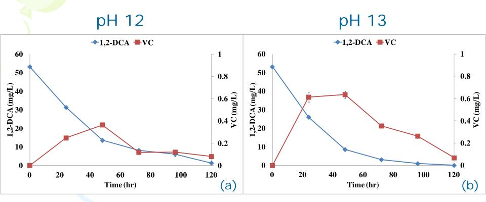
Fig. 2. Degradation of 1,2-DCA and production of VC during alkalineactivated PS oxidation (a) pH 12, (b) pH 13.
