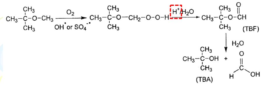
Fig. 6. Scheme of MTBE degradation with advanced oxidation processes Source: K.C. Huang et al., Chemosphere, 49,413-420, 2002
