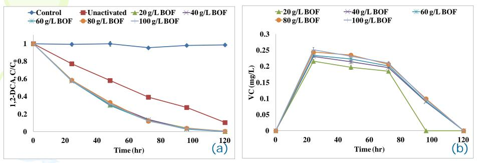
Fig. 7. Degradation of 1,2-DCA (a) and the production of VC (b) during PS oxidation with the addition of different dosages of BOF slag.
