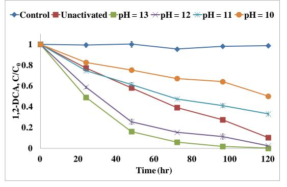
Fig. 1. 1,2-DCA removal by persulfate under different alkaline conditions
