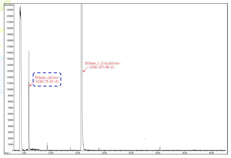
Fig. 3. Identification of VC production by GC-MS
