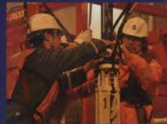
Long-term borehole thermometer installed in a borehole drilled by "CHIKYU" in the Japan Trench Fast Drilling Project (right), and its installation and its recovery (two photos on the left)
