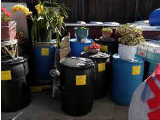
Photograph 7: Eight 55-gallon containers of hazardous waste without proper aisle space.
