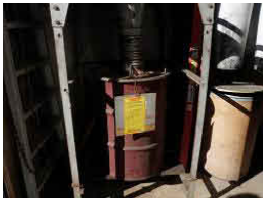
Photograph 3 : A picture of a 55-gallon drum of hazardous waste polishing dust that was improperly labeled in CA.
