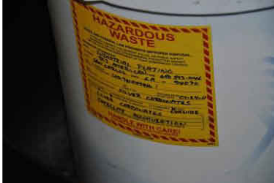
Photograph 2: The facility consolidated the two containers of silver waste into a third container that is closed and marked.
