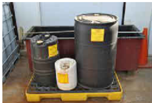
Photograph 17 : The opened poly-drum was closed and properly labeled.
