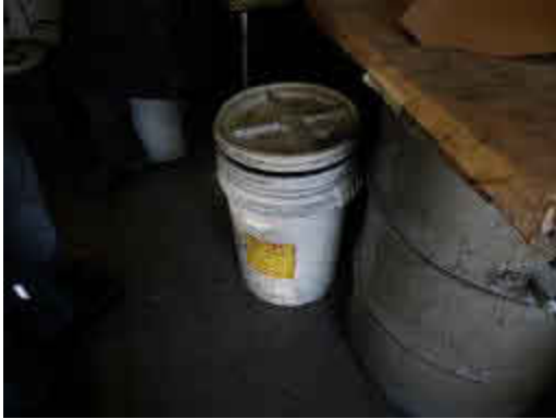
Photograph 5 : An open 5-gallon container of hazardous waste polishing dust. The label was not properly marked.
