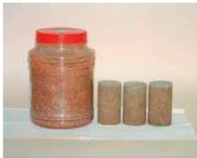
Figure 2. WOHEST was applied to deal with radioactive mixed IXR on bench scale
