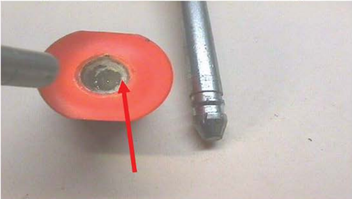
Glue inside locking mechanism. Seal does not lock properly.
