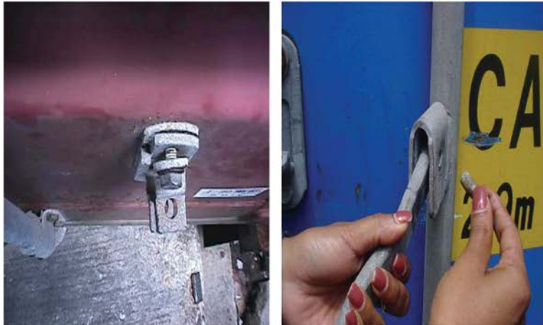
Detachable or loose bolts can allow access inside container
