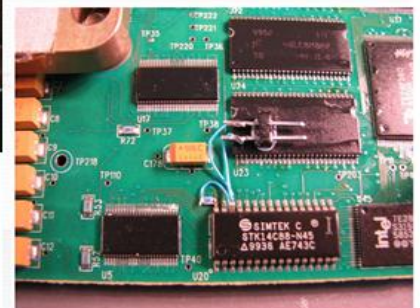
Figure 3-7 Close-up of CPU Board Modification to U20 Chip
