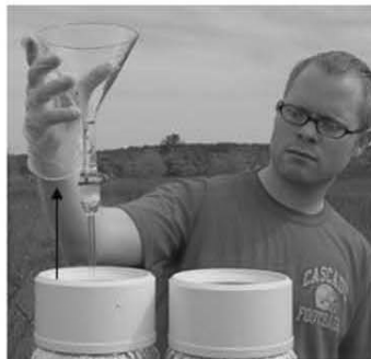
NCON: Removing funnel/sample train from chimney. (Notice how they are being carefully lifted straight up out of the collector.)
