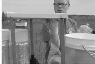
Cleaning lid seal as it cycles to cover the dry-side bag.
