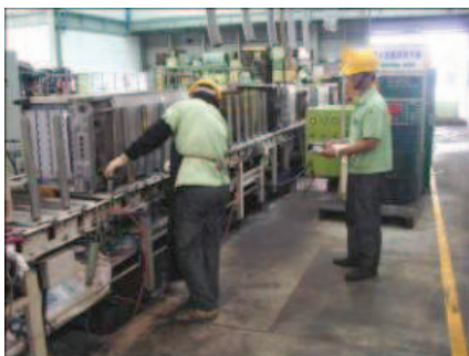
Extracting the refrigerant 冷媒抽取
