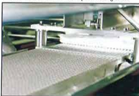
芯块自动装管/Automatic pellet loading device
