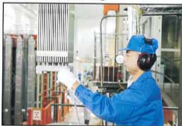
组件清洗/ FA cleaning
