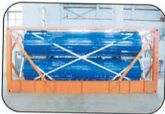
装有容器捆绑后的集装箱 Shipping container with bundled FA containers
