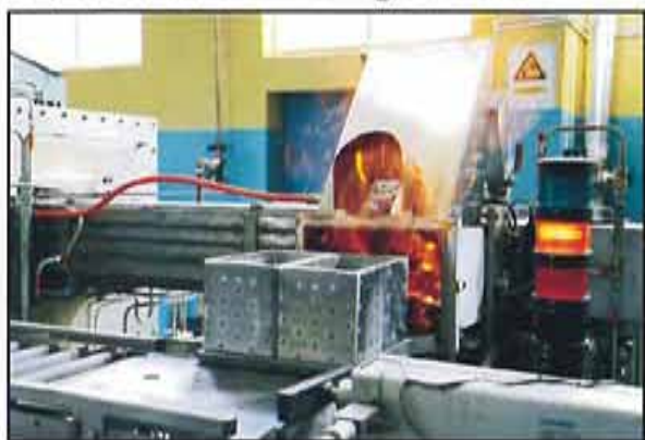
芯块烧结设备/ Sintering furnace
