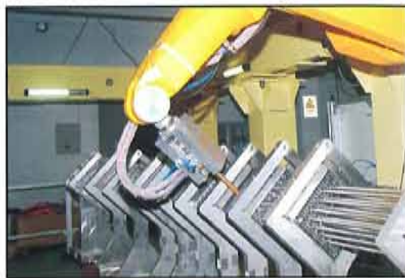
骨架焊接/ Skeleton welding
