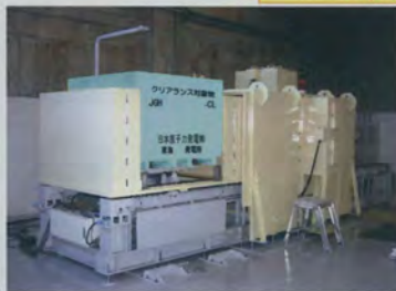
Clearance measurement equipment
