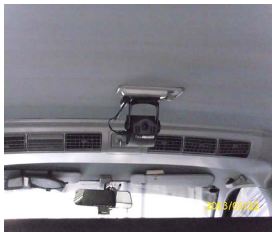
Figure 9. Dashboard cameras attached to a vehicle shipping the mobile radioactive sources
