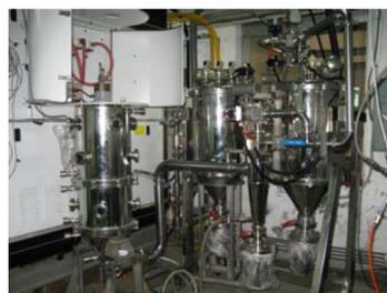
Figure 1. The photograph of the homemade ICP synthesis reactor and powder collection system.
