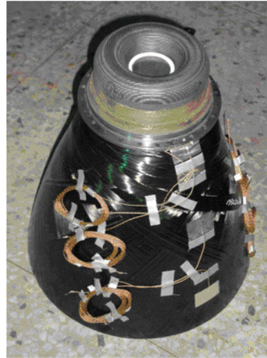
3D C/C nozzle with composite bell-shaped exit cone
