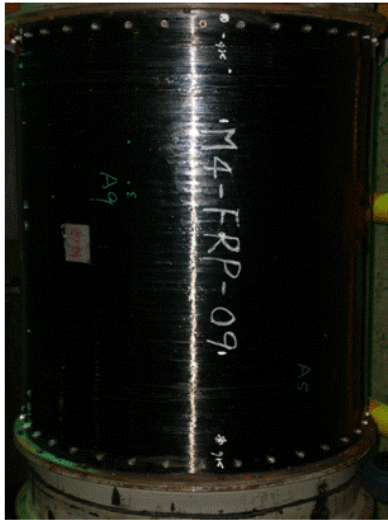
Carbon fiber motor case with metal flange
