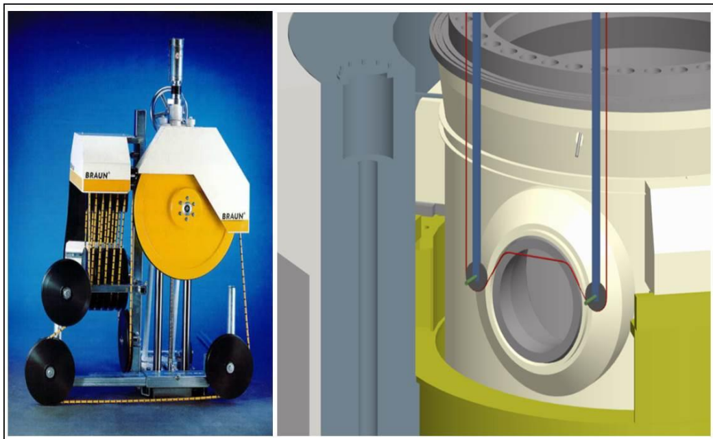
Diamond Wire Tool – Cutting of Nozzles
