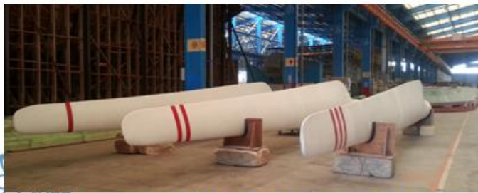
Blade(70% Glass fiber, 30% Carbon fiber)
