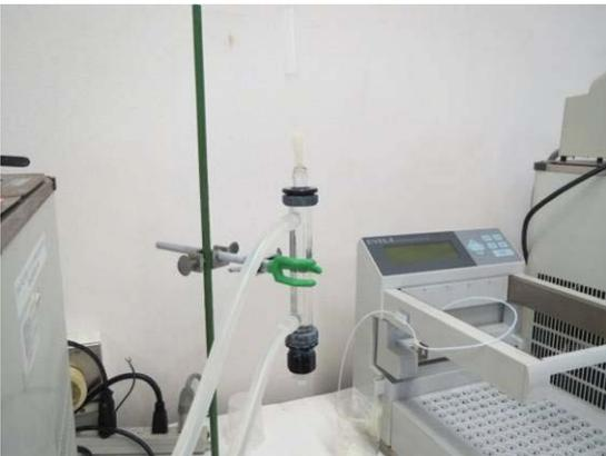
Loading TOA-MC (~0.5g) with DIW using pipette
