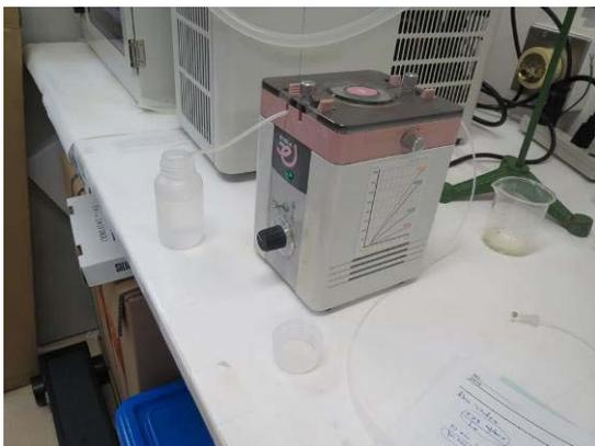
Fine-tuning using speed controller of peristaltic pump
