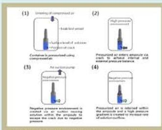
Figure 2 Inspection via pressurization and vacuum
