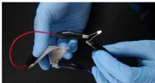
Fig. 2 Photo showing LED lamp-on with printed primary battery
