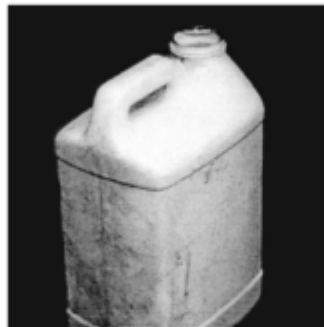
Figure 5 – Container with Dried Formulation that is Visible and Dislodgeable Residue. This Container is Unacceptable for Recycling. NOTE: To view a more accurate color rendition of Figure 5, a color photo of is available at http://www.asabe.org/standards/images/5596images.html
