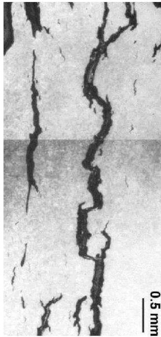
Multiple intergranular cracking in a 1CrMoV rotor which had run for 52,000h, with 190 starts [Skelton]
