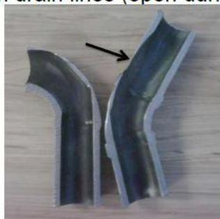
T91 main-steam drain-line after failure showing erosion from spalled oxides
