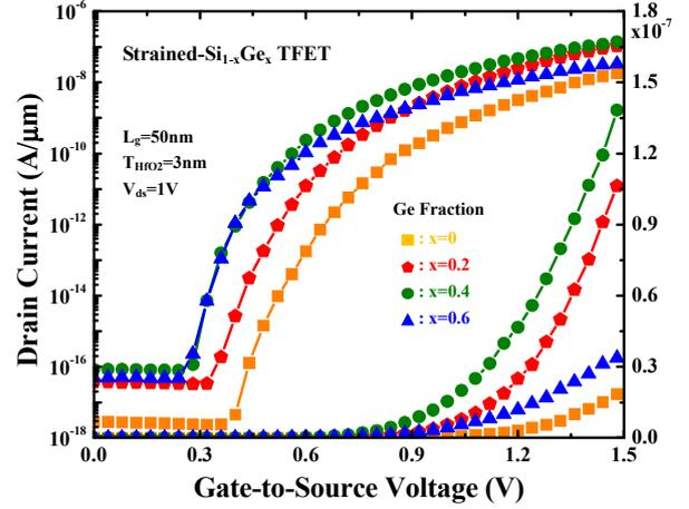
Fig. 6. Current-voltage curves of strained- $\text{Si}_{1-x}\text{Ge}_x$  double-gate TFETs with various Ge mole fractions.
