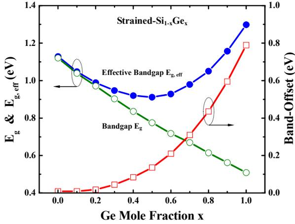
Fig. 4. Physical bandgap ( $E_g$ ), calculated band-offset and effective bandgap ( $E_{g,eff}$ ) of strained- $\text{Si}_{1-x}\text{Ge}_x$  in double-gate TFETs.
