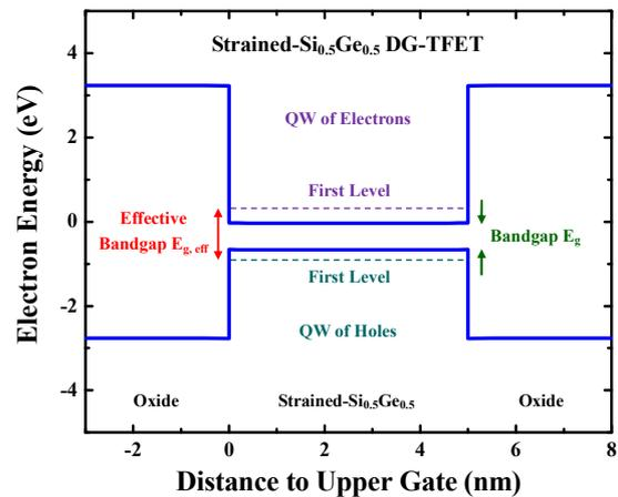
Fig. 3. Electrons and holes are confined in quantum wells in strained-Si<sub>1-x</sub>Ge<sub>x</sub> double-gate TFETs (x = 0.5 for illustration).
