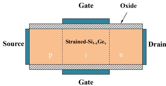
Fig. 1. Simulated structure of strained-Si<sub>1-x</sub>Ge<sub>x</sub> double-gate TFETs.
