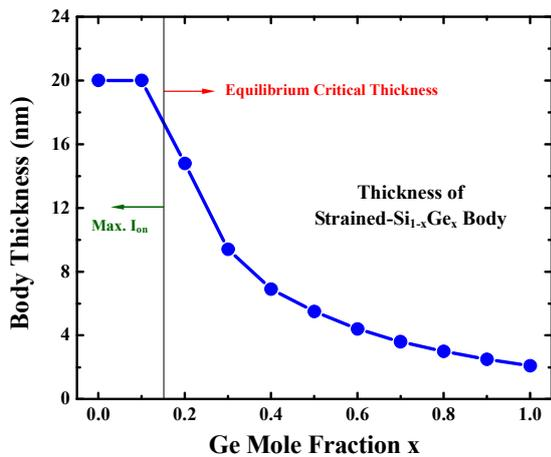
Fig. 2. Thickness of strained-Si<sub>1-x</sub>Ge<sub>x</sub> body used in double-gate TFET s with various Ge mole fractions from 0 to 1.
