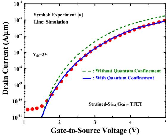
Fig. 5. Simulated current-voltage curves with and without including quantum confinement effect in comparison with experimental data of strained- $\text{Si}_{0.43}\text{Ge}_{0.57}$  TFETs [6].
