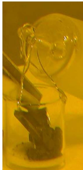
Leaching of fragments and cladding (Studsvik)
