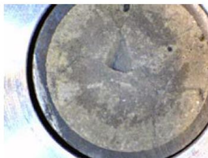
Cladded SNF pellet (KIT)
