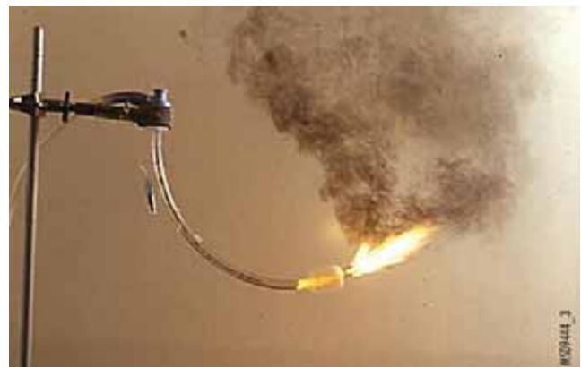
Demonstration of a burning tracheal tube with oxygen flowing through it. Note the flame and smoke being emitted from the tube, as well as the fire progressing inside the tube against the flow of oxygen.
