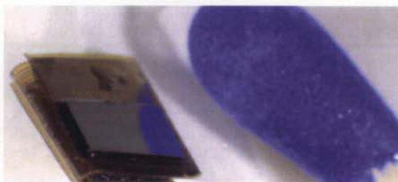
(c) 可撓曲軟膜晶片(Signal processing, wireless interface)：可用於超微型助聽器 (ultraminiature hearing aids)
