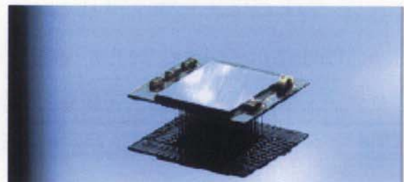
(b) 神經介面 (Sensor/Actuator, Antenna, RFInterface, Signal Processing, Power)：可用於義肢 (prostheses)
