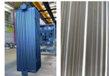
Radiator with homogenous CDC coating
