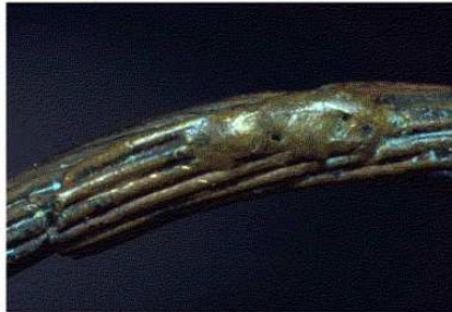
Exhibit 1-3029, from 10 AWG Left Emergency AC Bus Feed (magnification X10)
