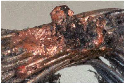
Exhibit 1-14723, from 12 AWG IFEN Power Cable (magnification X22)
