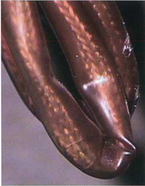
Improper Bend Radius
