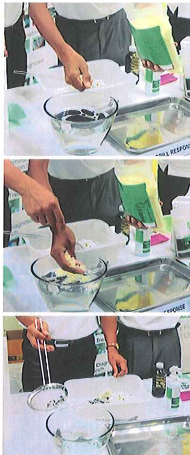
A demonstration shows the efficiency of Hi-Grimm's Keen line of oil-degrading bacteria. An oil spill is simulated (top), Keen microorganisms are sprinkled in (centre), and the oil is rapidly broken down (bottom).
