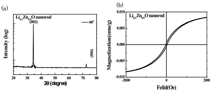
Figure 1. (a) XRD pattern of Li doped ZnO nanorods. (b) Magnetization and magnetic field curve of prepared samples.
