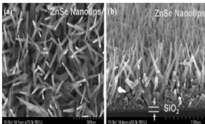
Fig.1(a) top view and (b) cross-sectional FESEM images of the ZnSe nanotips
