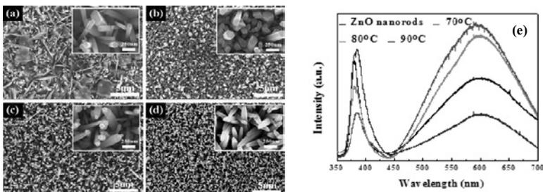
Fig 1. (a), (b), (c) top-view FESEM image of the Ga-doped ZnO nanorods grown at 70°C, 80°C, and 90°C and (d) un-doped ZnO nanorods. Inset in all top-view shows an enlarged FESEM image. (e) Room-temperature PL spectra of the un-doped ZnO and Ga-doped ZnO nanorods.
