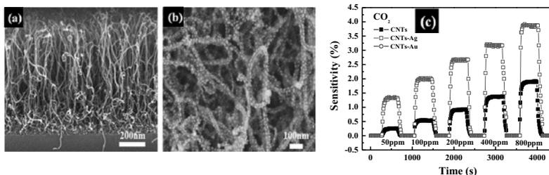
Fig. 1 (a) Cross-sectional and (b) high-magnification top-view FESEM images of the Ag-CNTs grown on Si substrate. (c) Sensor response of our Ag-CNT CO<sub>2</sub> gas sensor measured at various concentration.
