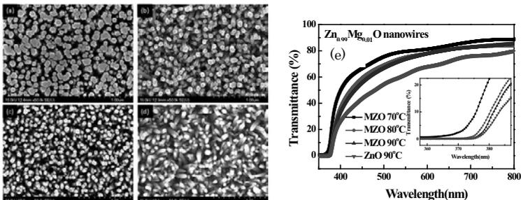
Figure 1. The top-view FE-SEM image of the (a) ZnO nanowires at 90°C and (b), (c), (d) show the Mg-doped ZnO nanowires grown at 70°C, 80°C, and 90°C, respectively. (e) The UV Spectrum of the ZnO and Mg-doped ZnO nanowires.
