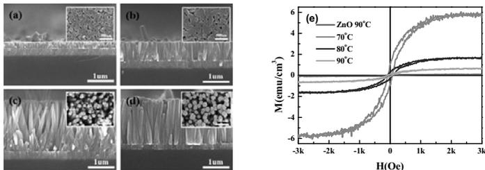
Figure1. (a), (b), (c), (d) shows FESEM image of the Ni-doped ZnO grown at 70°C, 80°C, 90°C, and un-doped ZnO nanorods at 90°C, respectively. Magnetic field curve loops of Ni-doped ZnO nanorod at room temperature.
