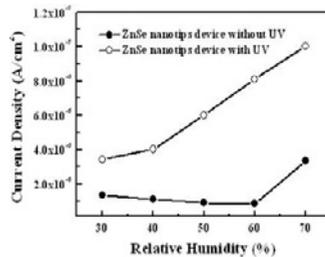
Fig. 2 Comparing UV illumination I-RH characteristics of ZnSe nanotips devices
