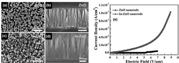
Fig. 1 (a) and (c) top-view FESEM image, (b) and (d) cross-sectional of the pure and indium doped ZnO nanorod grown on glass substrate, respectively. (e) Field emission characteristics of pure and indium-doped ZnO nanorods.
