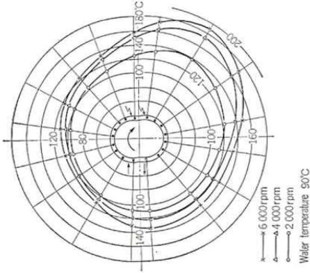
Fig. 3.5 Temperature distribution of inner surface of rotor housing
