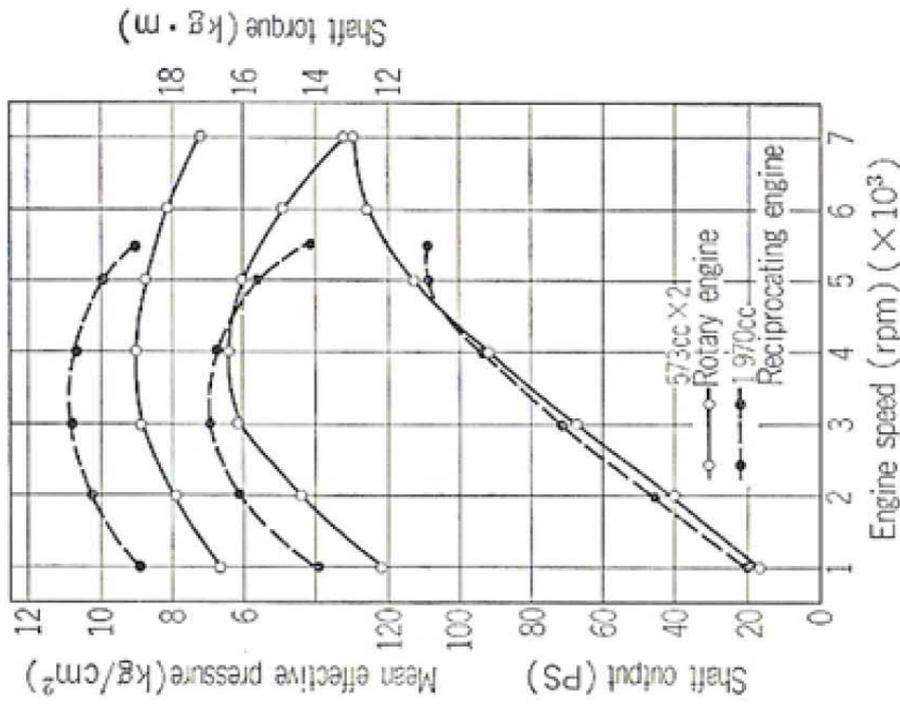
A comparison with a reciprocating engine shows a similar power at low speed with an increase high speed power.
