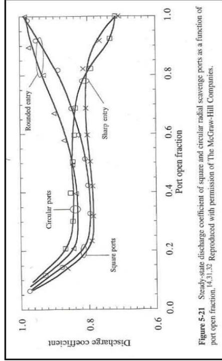
Figure 5-21 Steady-state discharge coefficient of square and circular radial scavenge ports as a function of port open fraction, 14,31.32. Reproduced with permission of The McGraw-Hill Companies.
