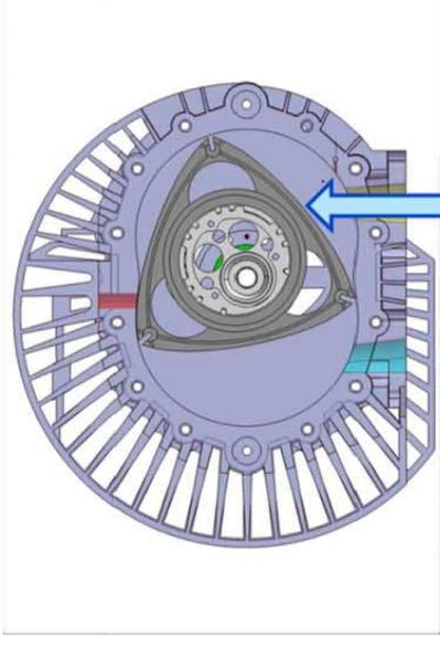
Inlet flow impinges on the rotor face
