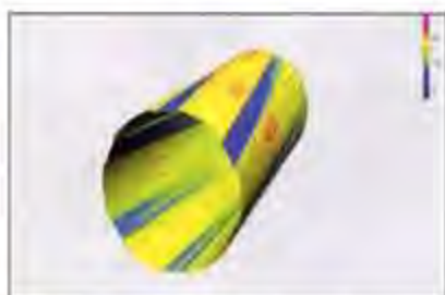
3D Image of Gun Barrel Rifling and Erosion
