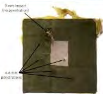
A 4.6mm steel ball round will penetrate a CRISAT target (the equivalent of a Soviet special forces bullet-proof vest) at 200 meters.
