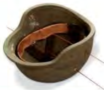
Kevlar helmet penetrations at 200 meters. The same 4.6 mm cartridge easily passes through automobile windshields with minimal deflection.
