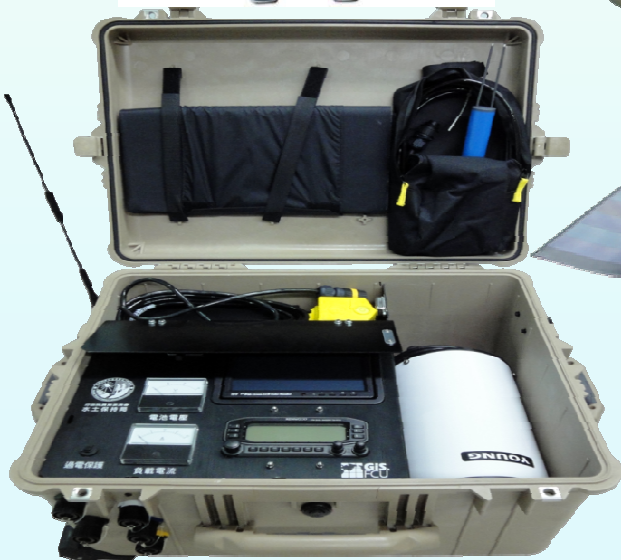
Data logger and battery
