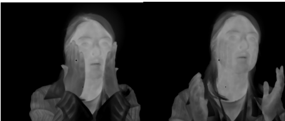
Figure 7: Images taken by the LWIR SLS based FPA (77 K).
