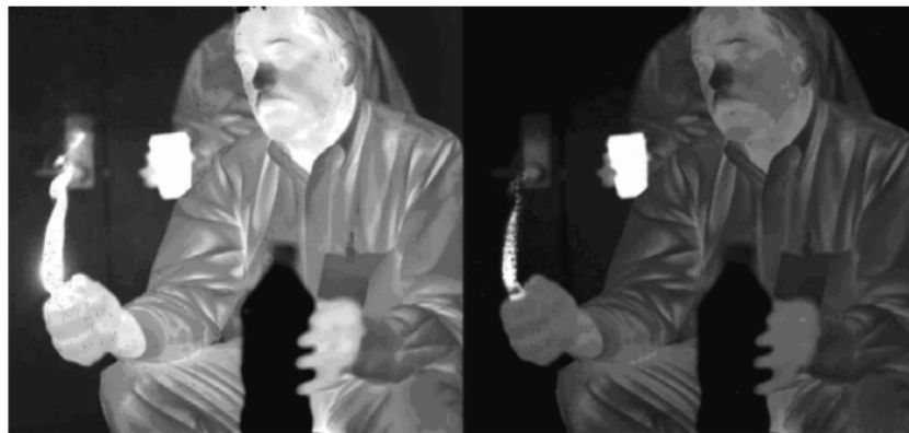
Fig. 10. An image taken with the first megapixel simultaneous pixel co-registered MWIR:LWIR dual-band QWIP camera. The flame in the MWIR image (left) looks broader due to the detection of heated CO 2 (from cigarette lighter) re-emission in 4.1–4.3-micron band, whereas the heated CO 2 gas does not have any emission line in the LWIR (8–9 microns) band. Thus, the LWIR image shows only thermal signatures of the flame.
