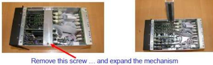
Remove this screw ... and expand the mechanism
