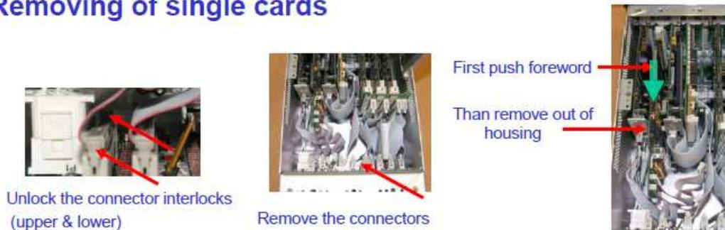
Unlock the connector interlocks (upper & lower)
