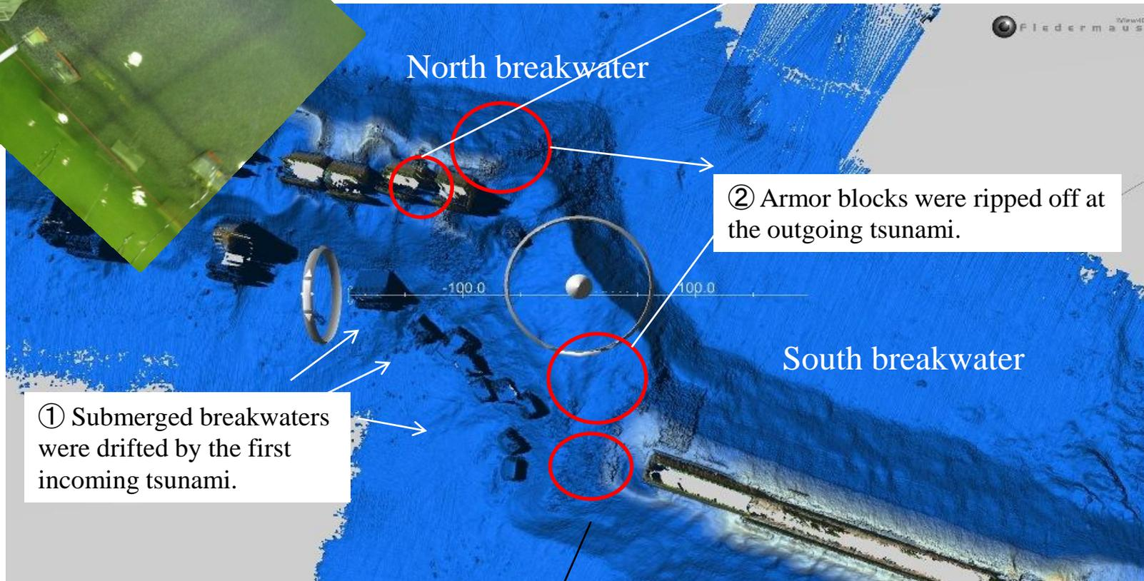
Although the mound was scoured, the head breakwater was not tilted.
