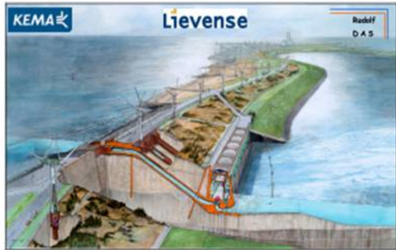
Fig. 4 – Concept of the Energy Island with an inverse pump accumulation system (IOPAC).
