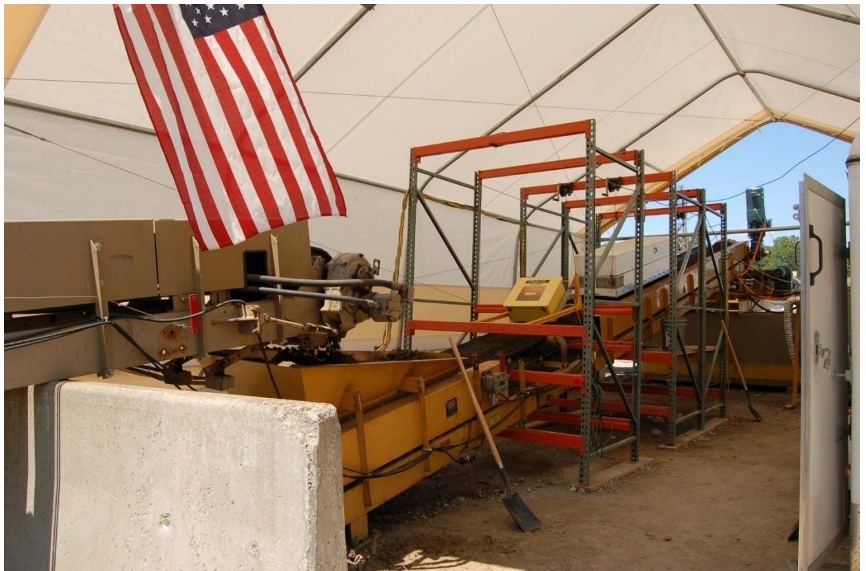
Figure 2 Survey Conveyor and Environmentally Controlled Detector Box (White)
