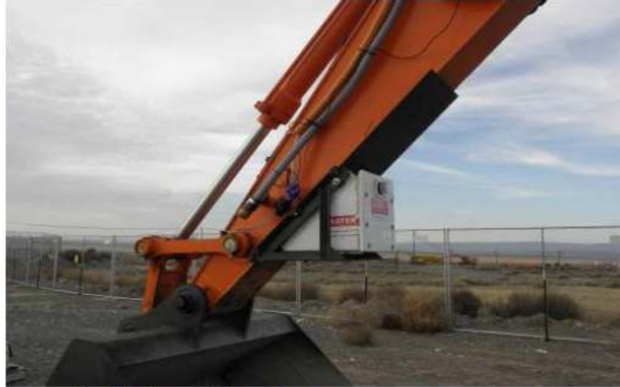
Redesigned Brackets on Excavator Boom
