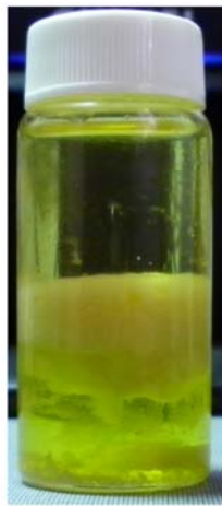
Figure 4 Another picture showing different layers of extracts of bitter almonds using ISFE.
