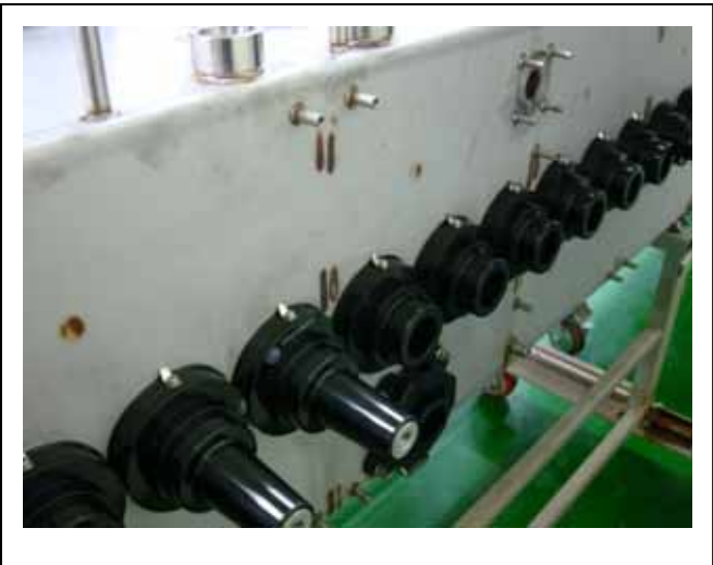
鎖緊套管及套管井接地簧片
