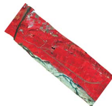
Self-calibrated DG rectified ISIS images in 1.0m ground resolution (2998 lines x 3133 pixels)
