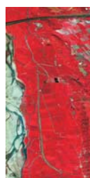
Raw ISIS images in 1.16m ground resolution (2250 lines x 1150 pixels; Red: \lambda_{182}=869.9\text{nm} , Green: \lambda_{94}=654.6\text{nm} , Blue: \lambda_{52}=551.9\text{nm} ).
