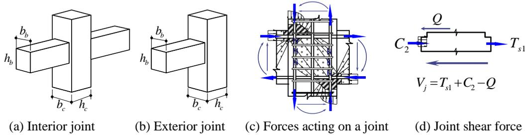
Figure 1. Terminology and forces acting on a joint under lateral loads
