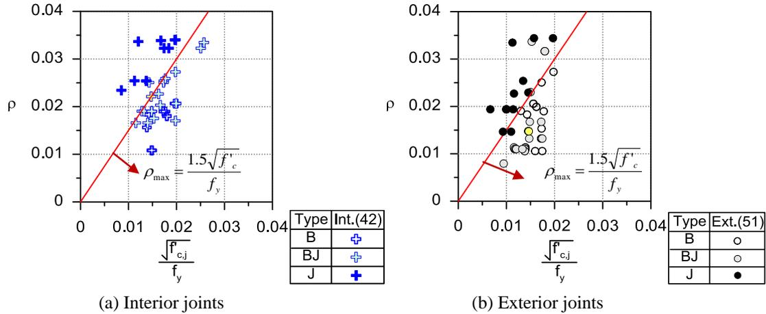
Figure 5. Maximum tensile reinforcement ratios for beams to preclude J-type failures
