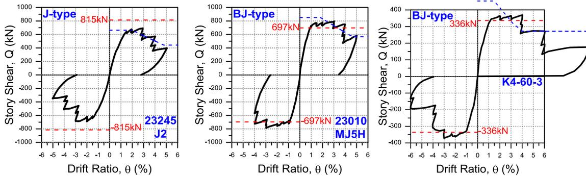
Figure 9. Comparison of proposed degradation model and test results (well-predicted cases)
