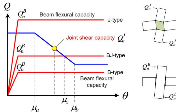
Figure 8. Illustrations for prediction of failure modes and ductility
