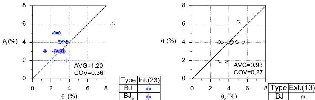
Figure 11. Comparisons of experimental-to-predicted story drifts
