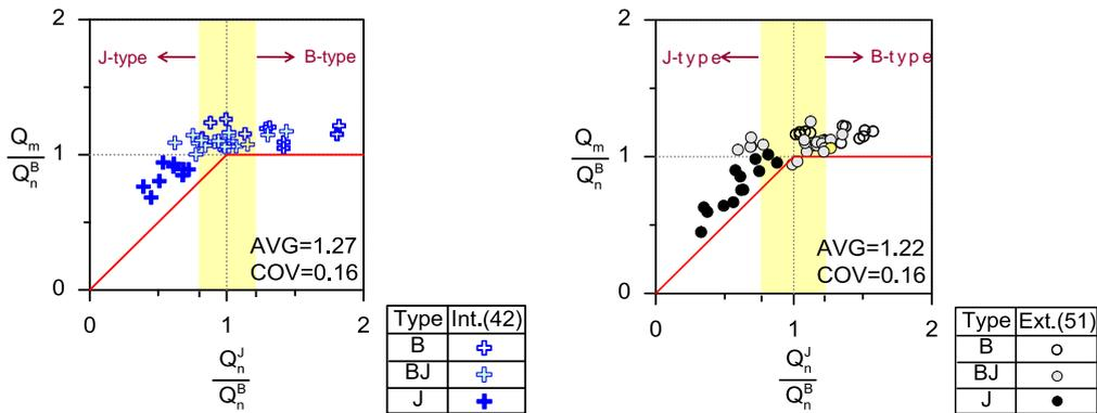
Figure 10. Comparisons of experimental-to-predicted story shear forces and failure modes
