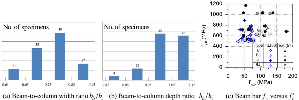
Figure 2. Range of aspect ratios and material strengths for the database
