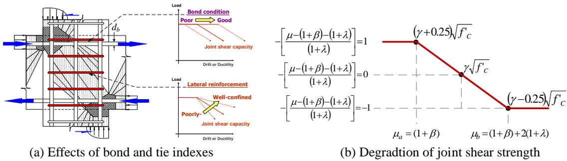
Figure 7. Proposed degradation model for joint shear strength with drift ductility
