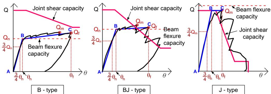
Figure 3. Definitions of yield drifts, failure drifts, and failure modes
