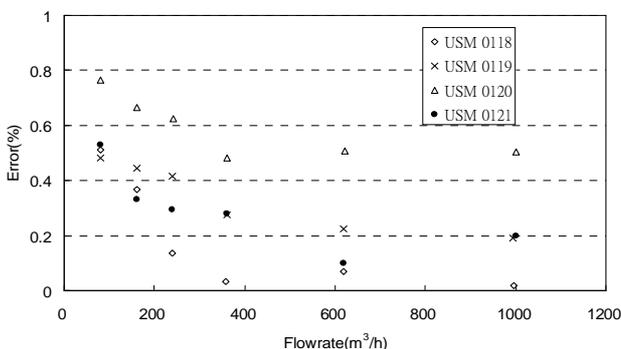
FIGURE 6. CALIBRATION DATA OF FOUR USM METERS AT WORKING PRESSURE: 10 KG/CM<sup>2</sup>
