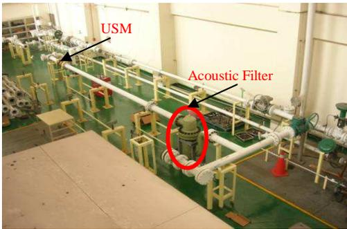
FIGURE 5. PIPE ARRANGEMENT OF USM CALIBRATION
