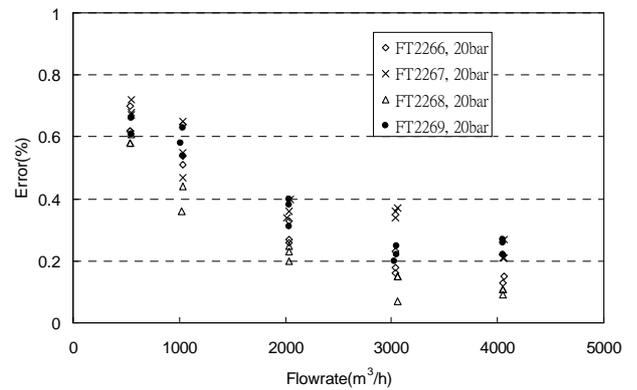
FIGURE 8. DATA OF 300MM USM CALIBRATION AT 20 KG/CM<sup>2</sup>
