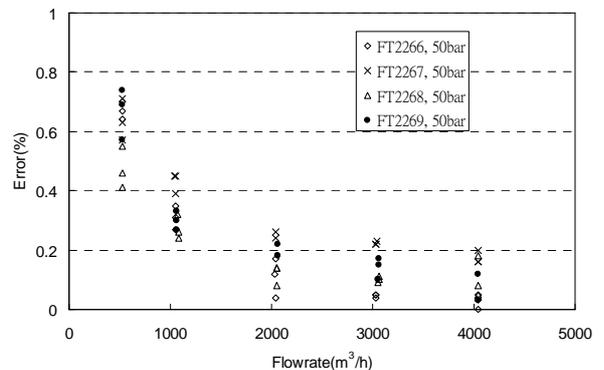
**FIGURE 9. DATA OF 300MM USM CALIBRATION AT 50 KG/CM<sup>2</sup>**
