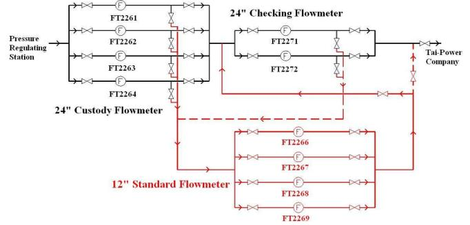
**FIGURE 3. SCHEMATIC DIAGRAM OF DA-TAN METERING STATION**
