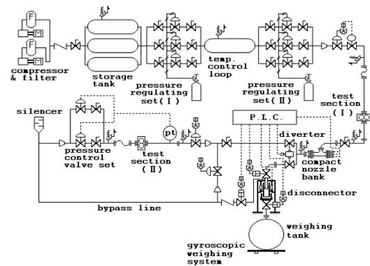
FIGURE 1. PRIMARY HIGH PRESSURE AIR FLOW MEASUREMENT STANDARD
