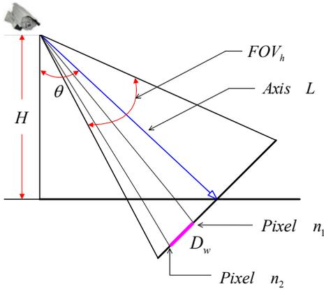
Fig. 3: The lateral distance estimation concept [23].
