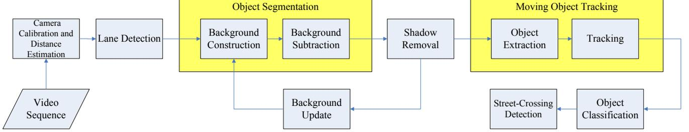
Fig. 1: Figure 1. Flowchart of the proposed automatic pedestrian and vehicle classification surveillance system for street-crossing safety.
