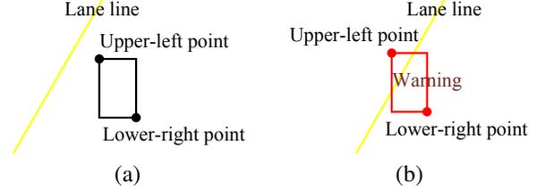
Fig. 6: (a) No warning signal is issued if the upper-left point and the lower-right point are on the same side of the street middle lane. (b) Lane-crossing violation is detected.
