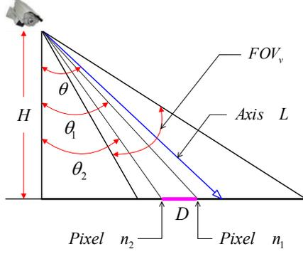
Fig. 2: The illustration of object longitudinal distance estimation [23].
