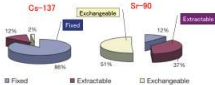
FIG. 3.18. Forms of radionuclides in soddy podzolic loam sand soil of the Gomel region of Belarus in 1998 [3.46].
