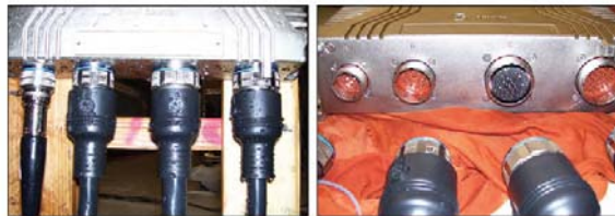
Figure 6. HardFiber Brick merging units tested for water ingress (pressure washing); post water inspection
