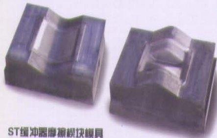
ST缓冲器摩擦楔块模具 Forging dies for the friction wedge of draft gear ST
