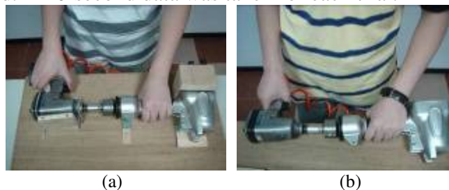
Figure 3. Subjects' typical posture in performing screw top fastening task (a) with and (b) without the fixture use
