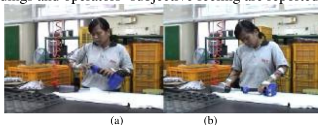
Figure 1. Work postures of an assembly operator while (a) installing a screw top at the handle butt and (b) tightening the screw top using an impact wrench
