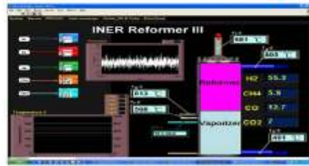
Compositions of reformat gas and its temperatures in a reformer
