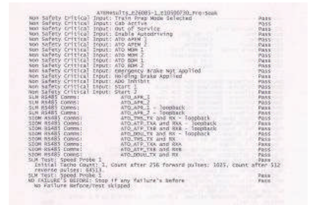
ATP 界面測試(RS-485 Pass)
