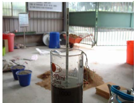
High concentration of sludge in the outflow at the beginning
